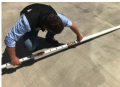
Figure 10- Sentek moisture probe with moisture meters
