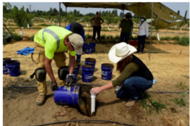
Figure 8 - Pouring Soil Slurry Backfill around Moisture Probe Casing (Thune 2021)
